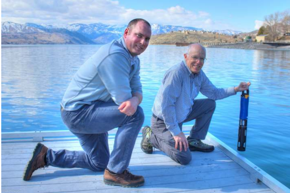
Dr. Long demonstrates the multiparameter probe that collects data every 15 minutes on temperature, conductivity, dissolved oxygen, turbidity, blue green algae and chlorophyll at Sunset Marina. Here Eric Campbell observes the measurements being taken adjacent to Campbell's resort.
